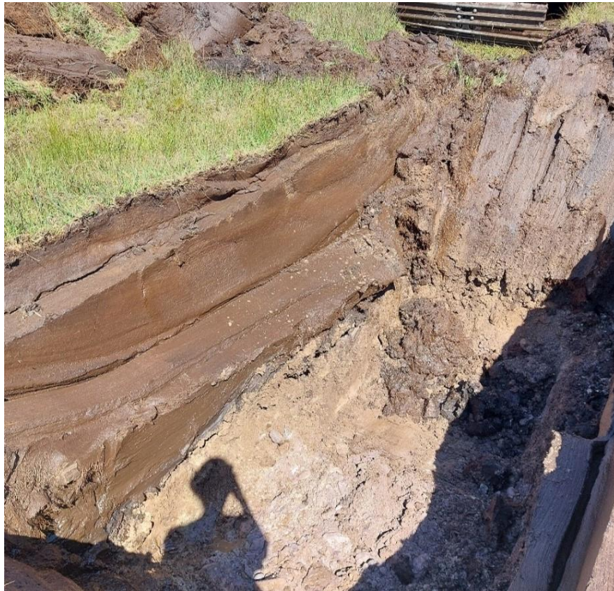
Figure 2-3: Photo of trial pit through peat and underlying weathered bedrock material at the proposed western temporary construction compound.
